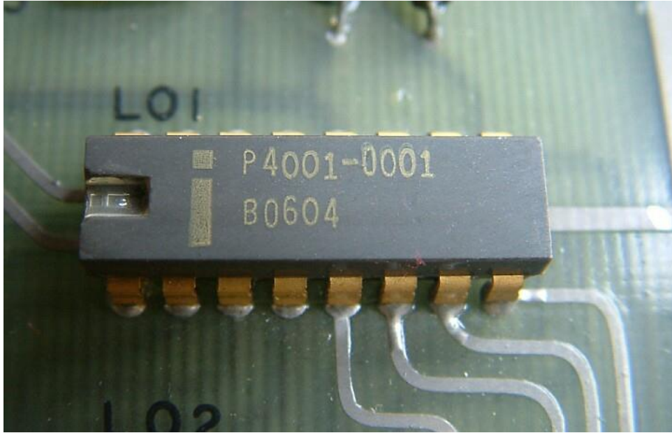
Intel P4001 with Yellow Logo and Part Number on Busicom 141-PF Main Board
